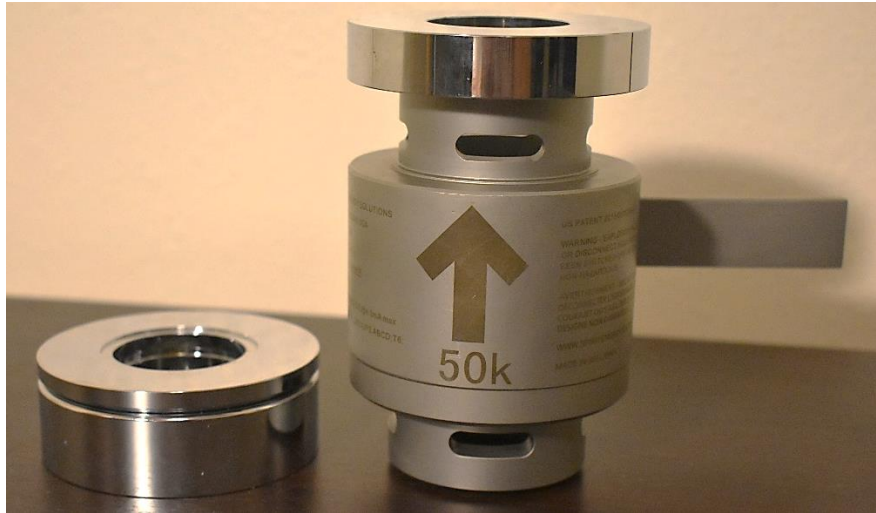
Fig. 38 Load Cell and Components
