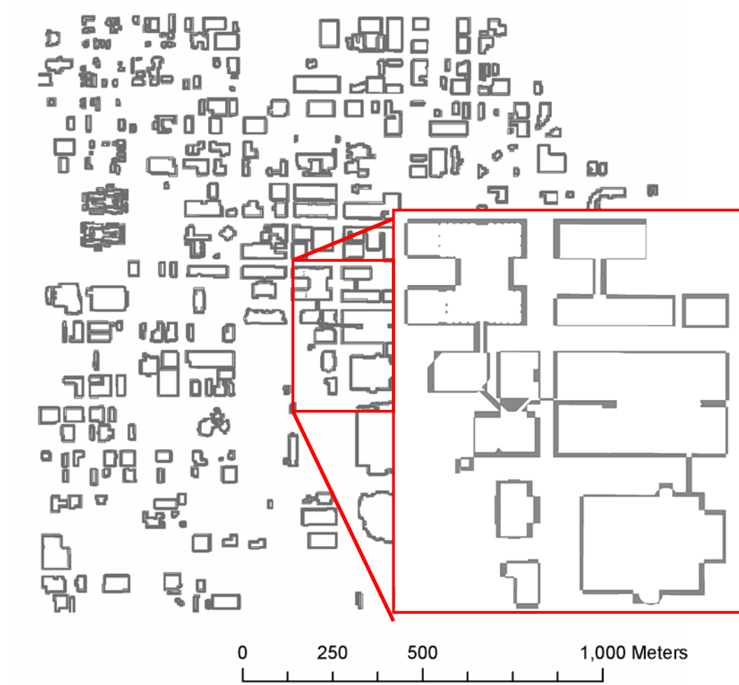
Figure 3.15. The spatial distribution of omitted and committed footprint area after conversion. Area in grey is a combination of omitted and committed footprint area at twelve meter resolution.
