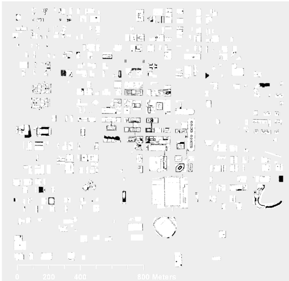
Figure 2.8. Area in black show potential LiDAR errors with more than 3 meters differences from the refined building model.
