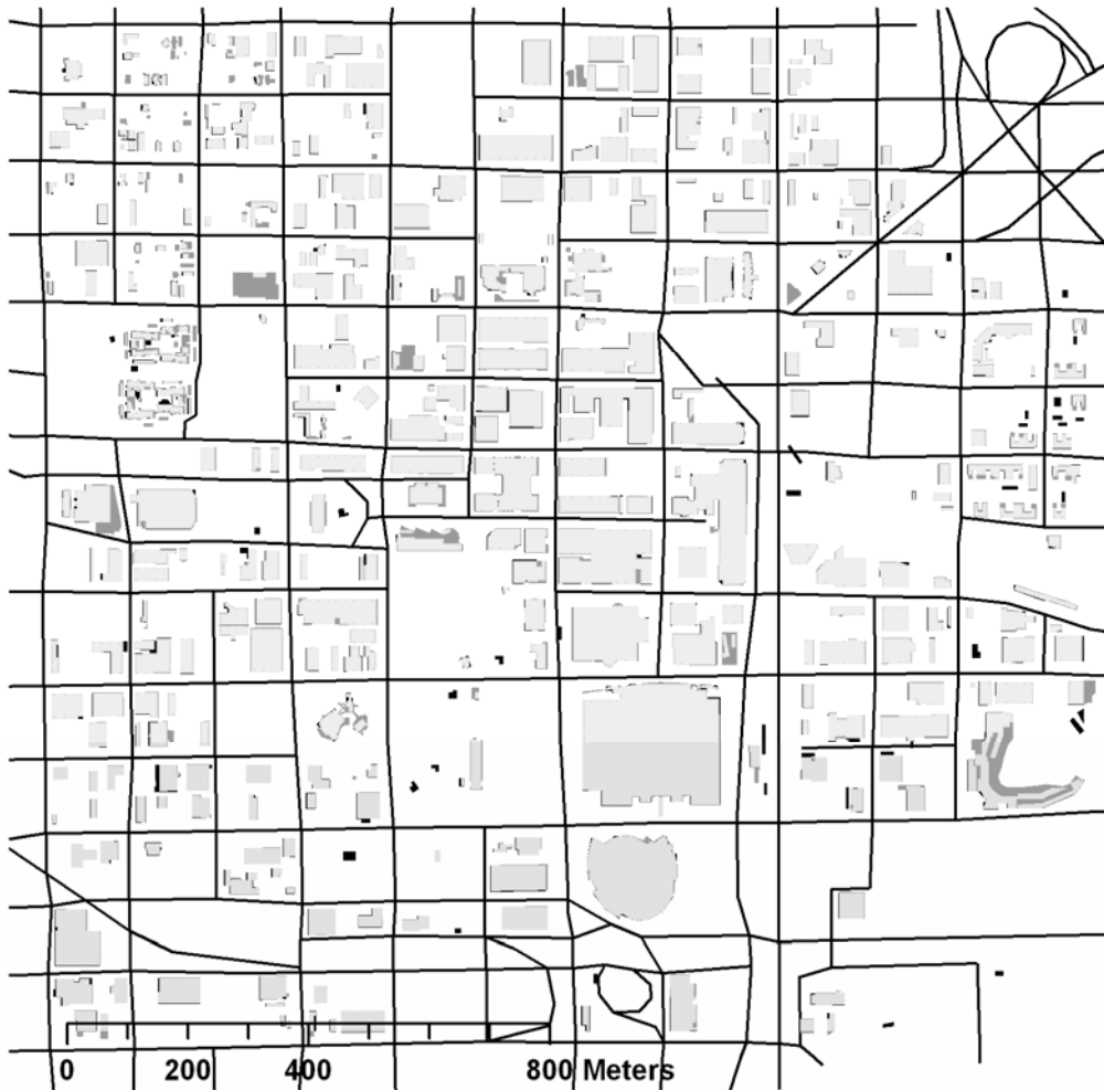
Figure 2.14. Overlay automatic building footprint with refined building footprint. Grey shows area of intersection; black shows area that are classified as building by algorithm but not by the refined model; medium-dark grey shows area that are classified as building by refined model but not the algorithm.
