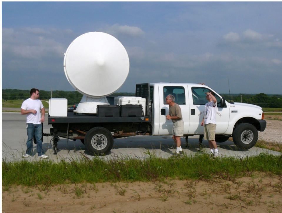
Fig. 11. The UMass X-Pol radar truck (in 2008) and its attendant crew members (C. Baldi, H. Bluestein, and J. Snyder). Photograph © R. Tanamachi.
