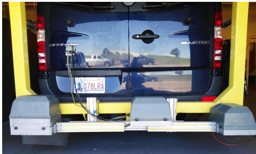
Figure 3.4. AMES 8300 High Speed Profiler
