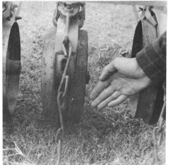
Figure 39. Close-up of Nesbit grass seeder showing planter boxes (left), and furrow opener disks with flanges (right) to prevent planting at excessive depths.
