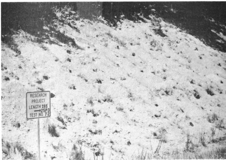
Fig. 30. A 45°, very highly erodible slope of Hector fine sandy loam on SH-1, in Le Flore county.
