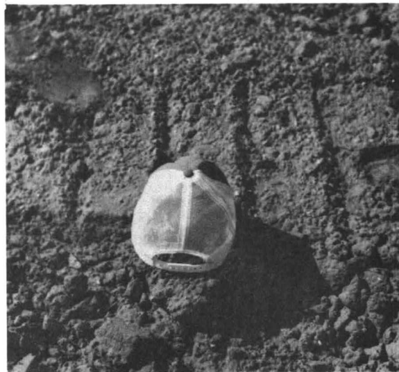
Figure 41. The usual smooth, compacted backslopes soil where an erosion resistant ground cover is to be established. (Note lug marks from a crawler tractor).
