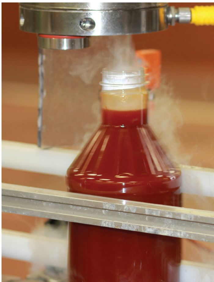
Nitrogen gas used as a processing aid in a barbecue sauce plant.
