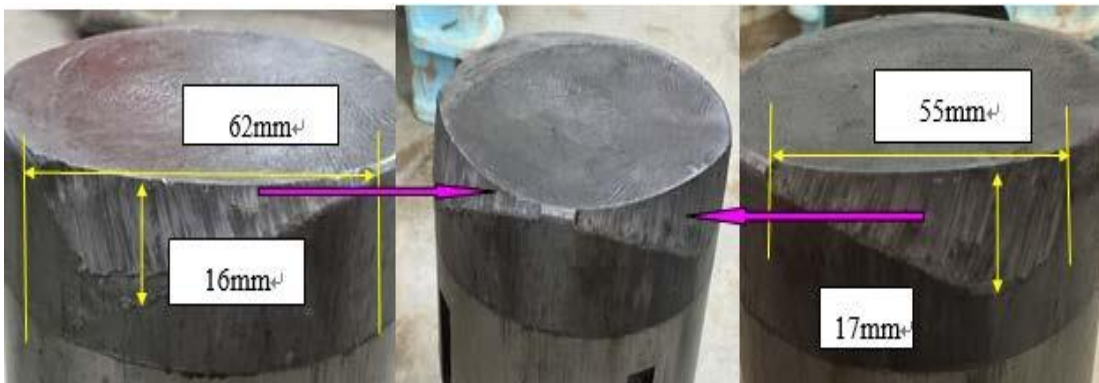
Figure 75. Picture of lead mold printing in deformed casing of well A-6
