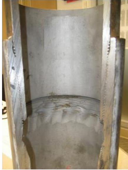
Figure 10. Eroded connection from field under hydraulic fracturing operations (Farahani et al., 2011)
