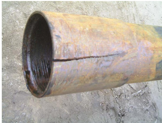
Figure 15. Connection failure (Magill, 2013)
