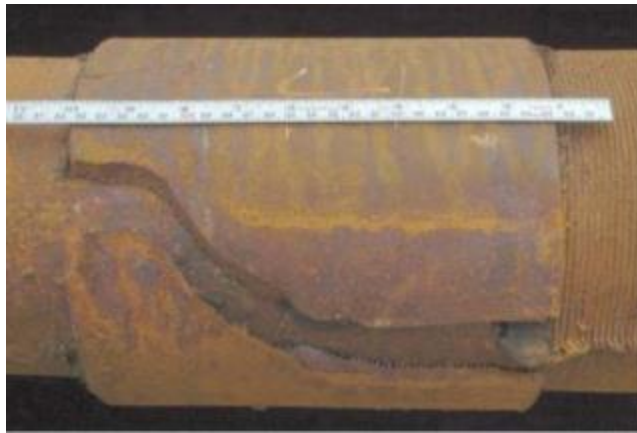
Figure 14. Coupling fatigue (Adams et al., 2017)
