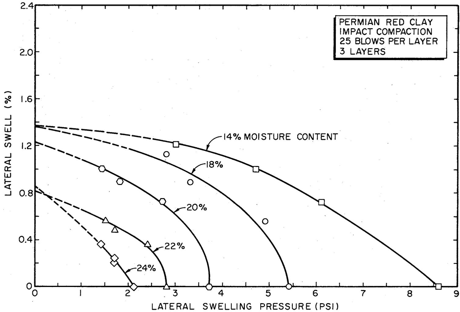
Figure 4.9. Effect of Lateral Swell on Lateral Swelling Pressure for PRC.
