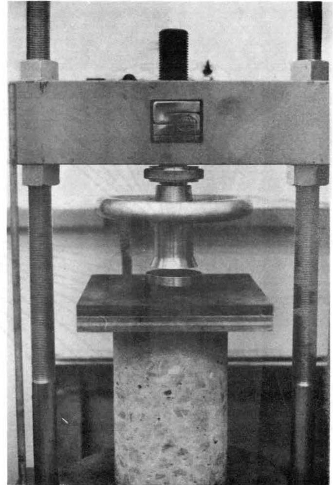
Figure 3.8. Compaction Equipment for Vertical Swelling Pressure Samples.
