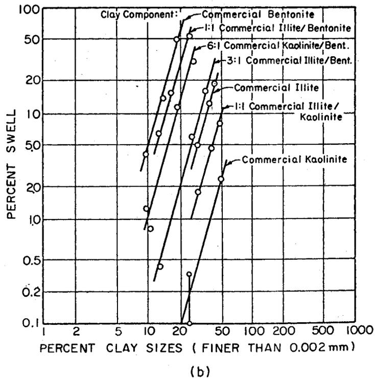
Figure 2.4. Relationship Between Percentage of Swell and Percentage of Clay Sizes for Experimental Soils: (a) Arithmetic Scale and (b) Logarithmic Scale (after Seed, Woodward, and Lundgren, 1962).
