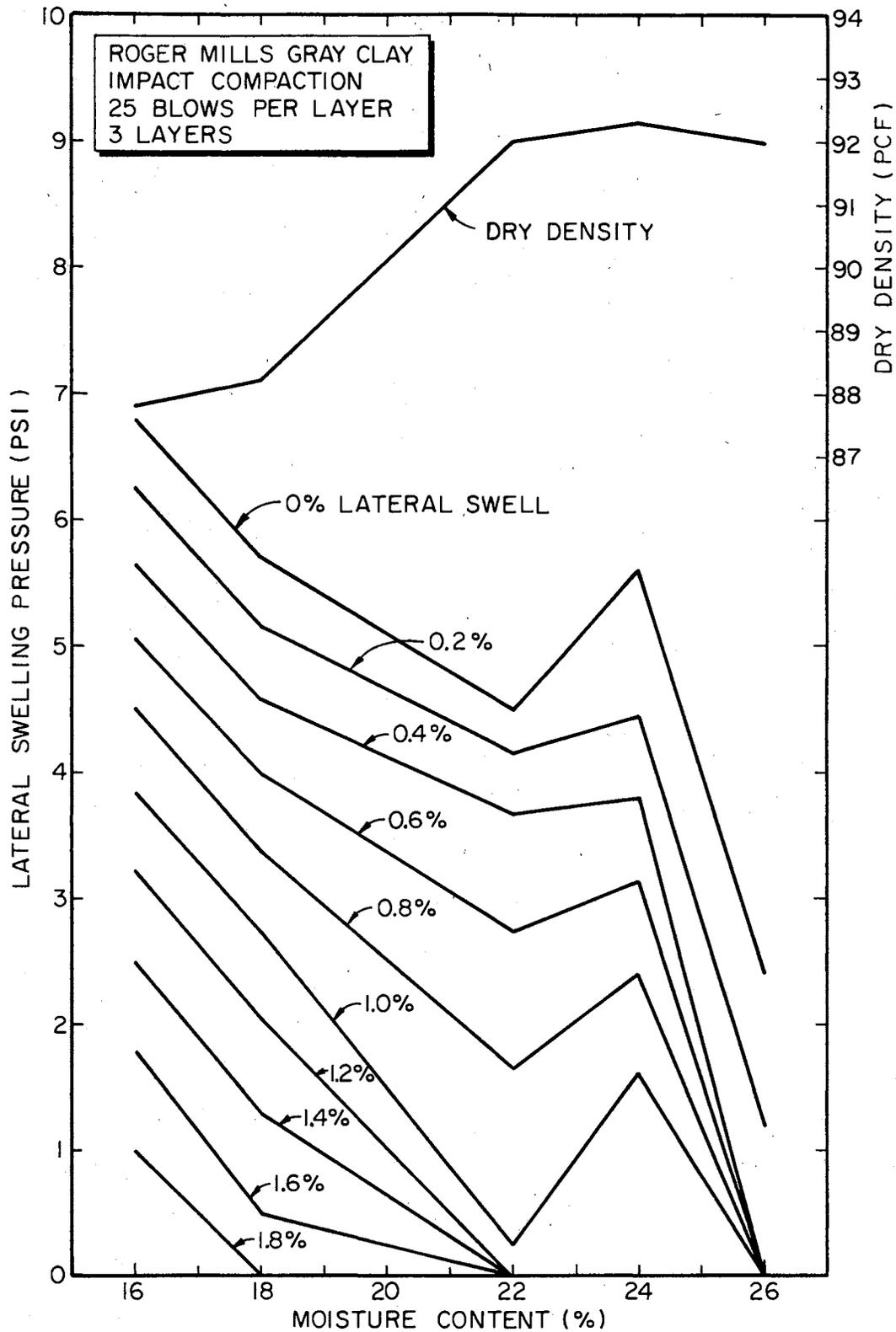
Figure 4.12. Effect of Initial Moisture Content on Lateral Swelling Pressure at Equal Percentages of Lateral Swell for RMGC.
