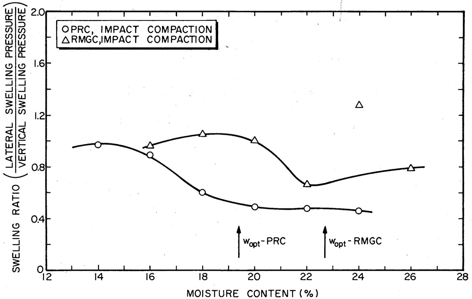
Figure 4.15. Effect of Initial Moisture Content on Swelling Ratio for PRC and RMGC.
