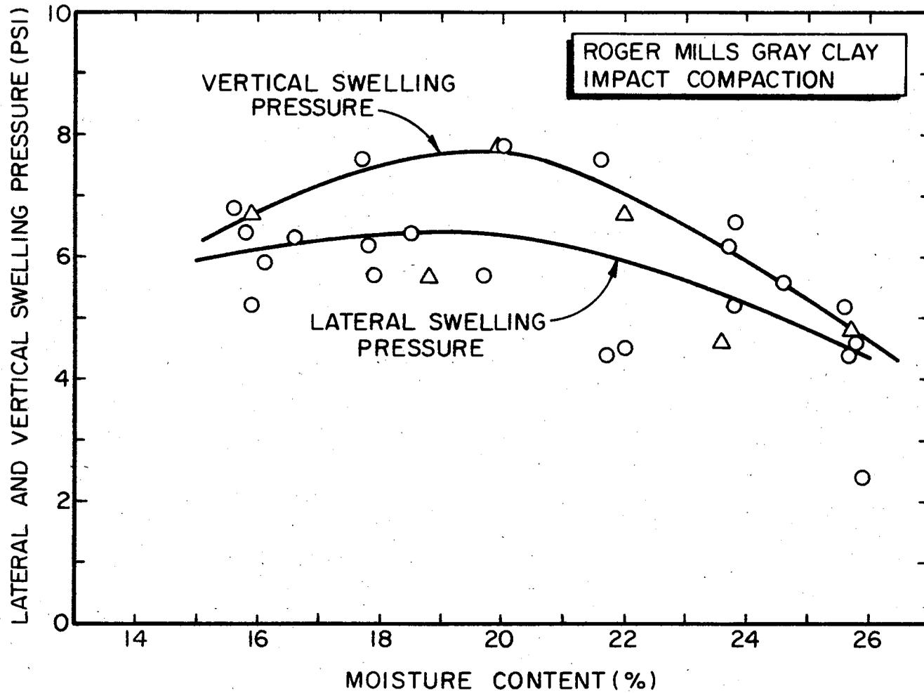
Figure 4.14. Lateral and Vertical Swelling Pressure versus Initial Moisture Content for RMGC.
