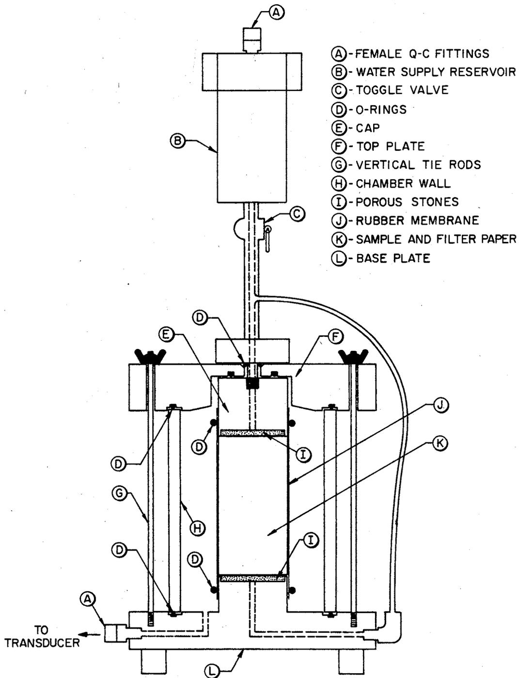
Figure 3.3. Diagram of Lateral Swelling Pressure Cell.
