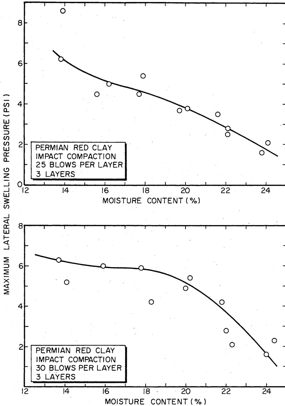
Figure 4.3. Effect of Initial Moisture Content on Lateral Swelling Pressure for PRC.
