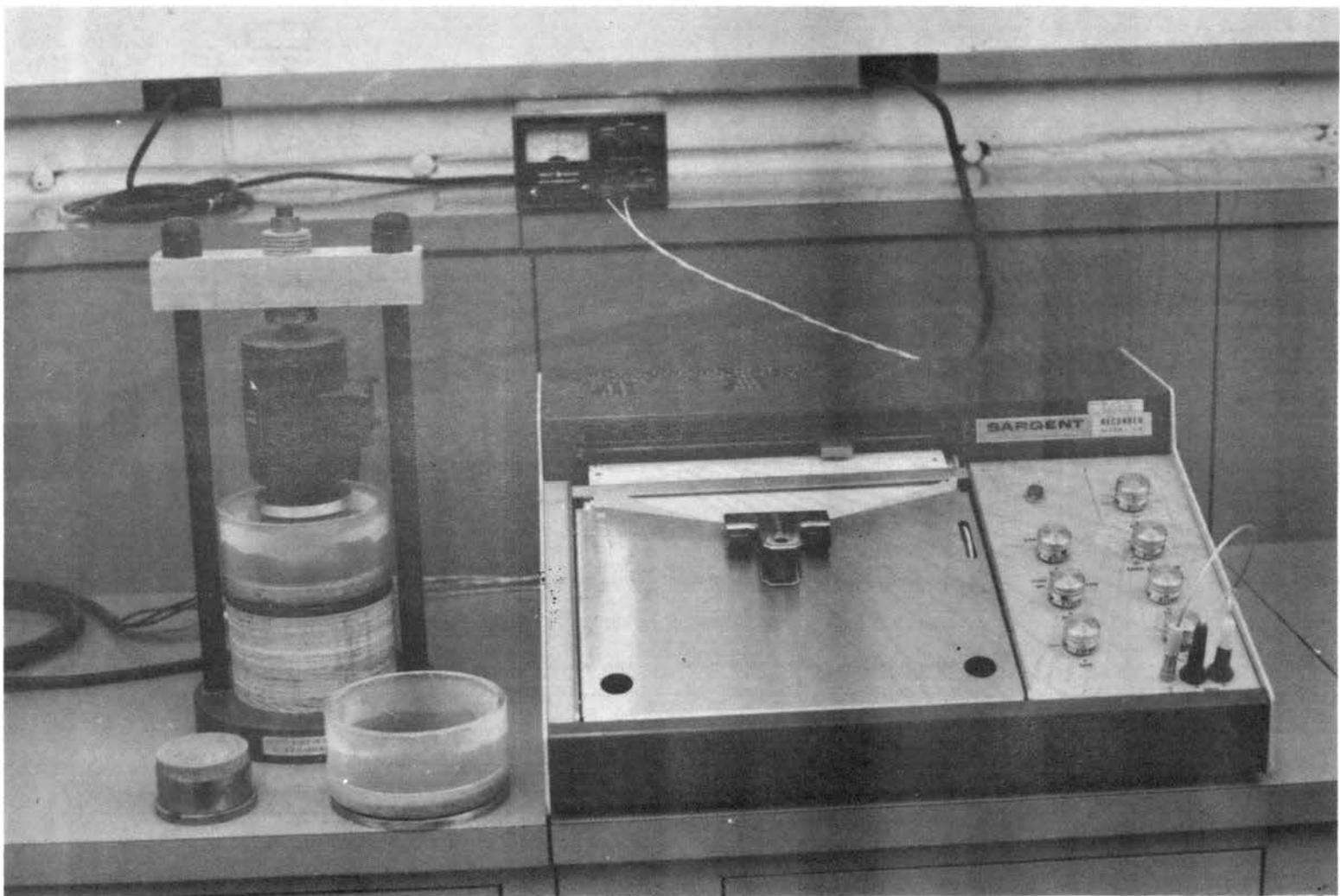
Figure 3.6. Test Assembly for Vertical Swelling Pressure Measurement.
