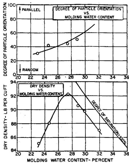
Figure 2.7. Influence of Molding Water Content on Particle Orientation for Compacted Samples of Kaolinite (after Seed and Chan, 1961).
