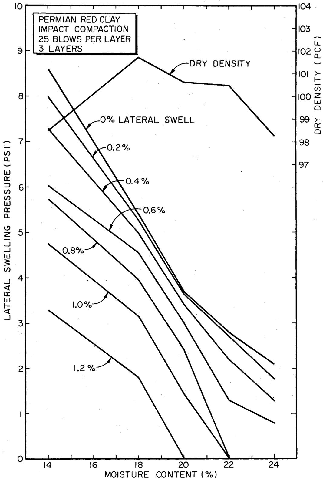
Figure 4.11. Effect of Initial Moisture Content on Lateral Swelling Pressure at Equal Percentages of Lateral Swell for PRC.
