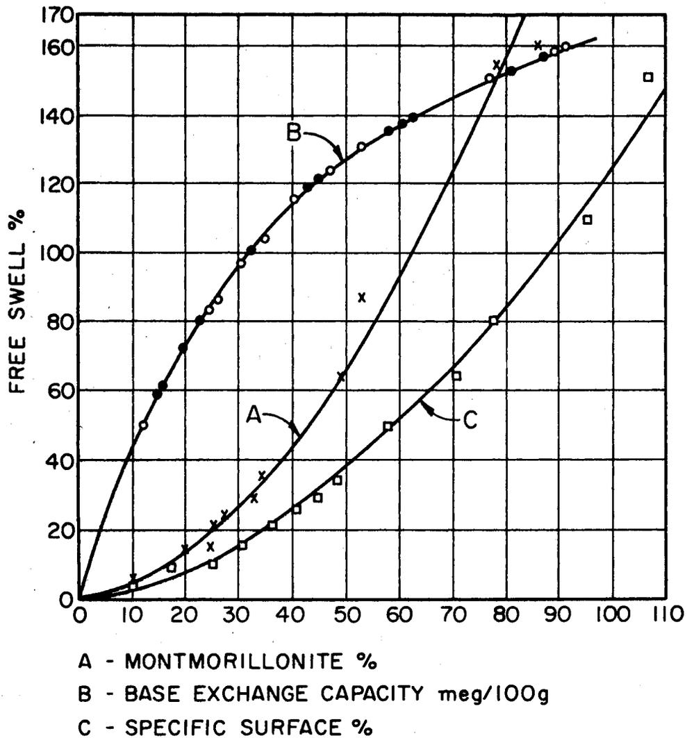
Figure 2.5. Free Swell versus Montmorillonite Content, Base Exchange Capacity and Specific Surface (after Gupta, Gupta, and Shukla, 1967).
