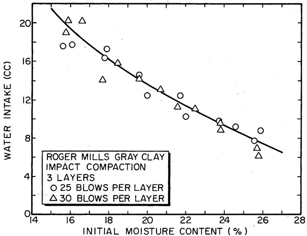
Figure 4.1. Water Intake versus Initial Moisture Content for PRC (upper) and RMGC (lower).
