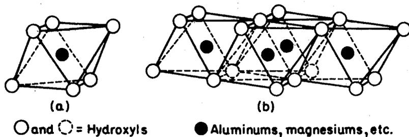
Figure 2.2. Diagrammatic Sketch Showing (a) a Single Aluminum Octahedron and (b) the Sheet Structure of the Aluminum Octahedrons (after Grim, 1968).
