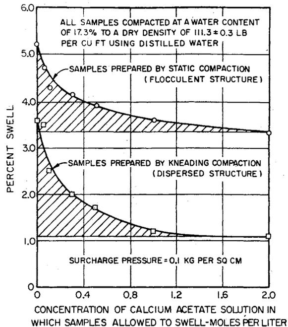
Figure 2.10. Effect of Structure and Electrolyte Concentration of Absorbed Solution on Swell of Compacted Sandy Clay (after Seed, Mitchell, and Chan, 1961).
