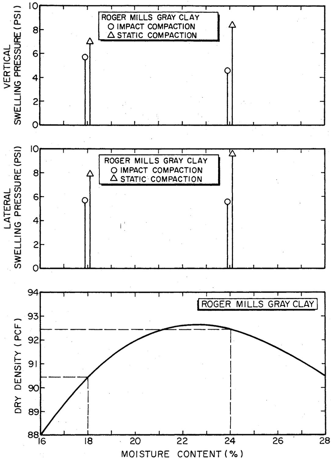
Figure 4.8. Effect of Compaction Method on Lateral and Vertical Swelling Pressure for RMGC.
