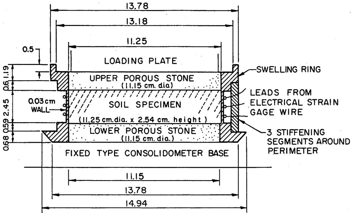
Figure 2.15. Swelling Pressure Ring for Lateral Swelling Pressure Measurements (after, Komornik and Zeitlen, 1970).
