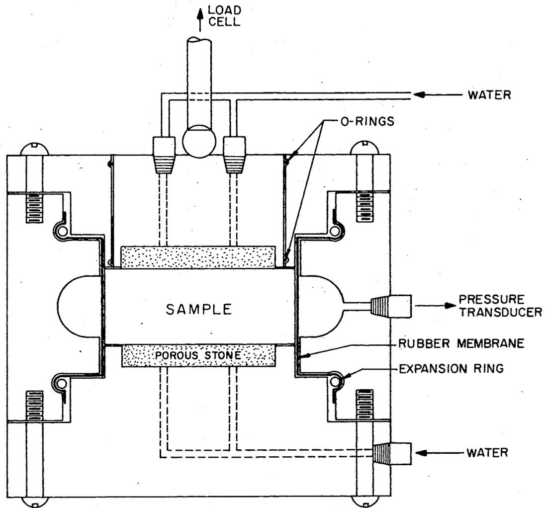
Figure 5.1. Suggested Device for Concurrent Measurement of Lateral and Vertical Swelling Pressure.
