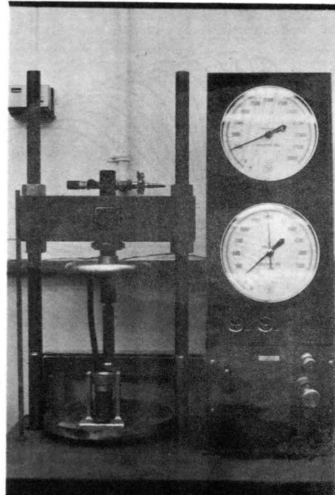
Figure 3.7. Compaction Equipment for Lateral Swelling Pressure Samples.
