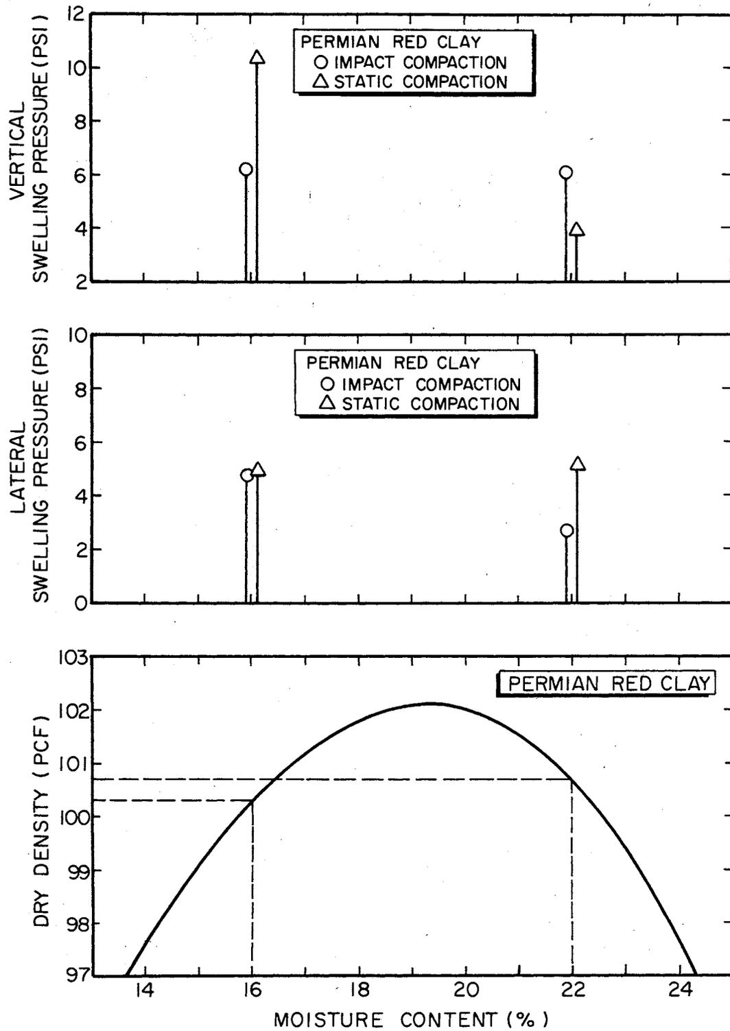
Figure 4.7. Effect of Compaction Method on Lateral and Vertical Swelling Pressure for PRC.
