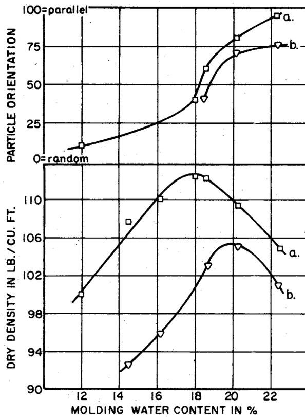
Figure 2.6. (a) Effects of Compaction on Soil Structure and (b) Particle Orientation versus Water Content for Boston Blue Clay (after Lambe, 1960).
