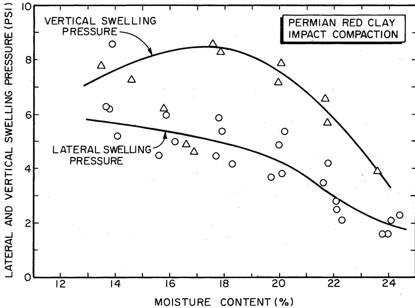
Figure 4.13. Lateral and Vertical Swelling Pressure versus Initial Moisture Content for PRC.
