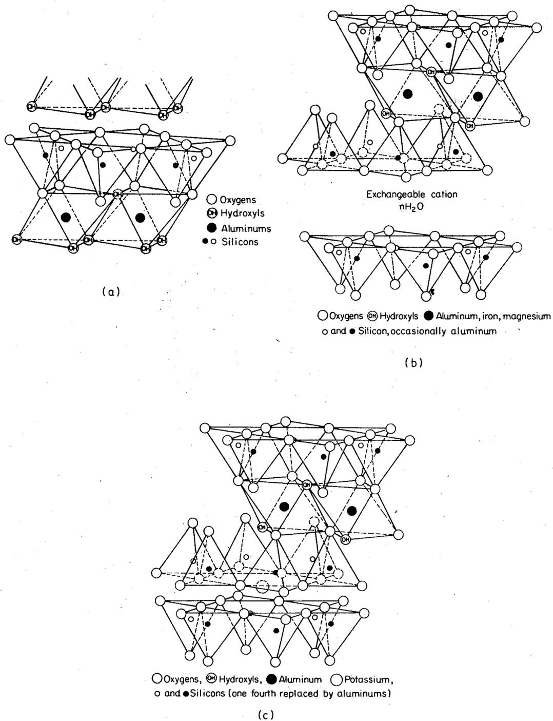
Figure 2.3. Structure of the Major Clay Mineral Groups: (a) Kaolinite; (b) Montmorillonite; and (c) Illite (after Grim, 1968).
