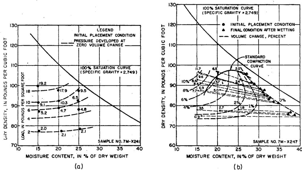
Figure 2.8. (a) Total Uplift Pressure for Various Placement Conditions and (b) Percent Expansion for Various Placement Conditions for Soil Under 1 psi Load (after Holtz and Gibbs, 1956).
