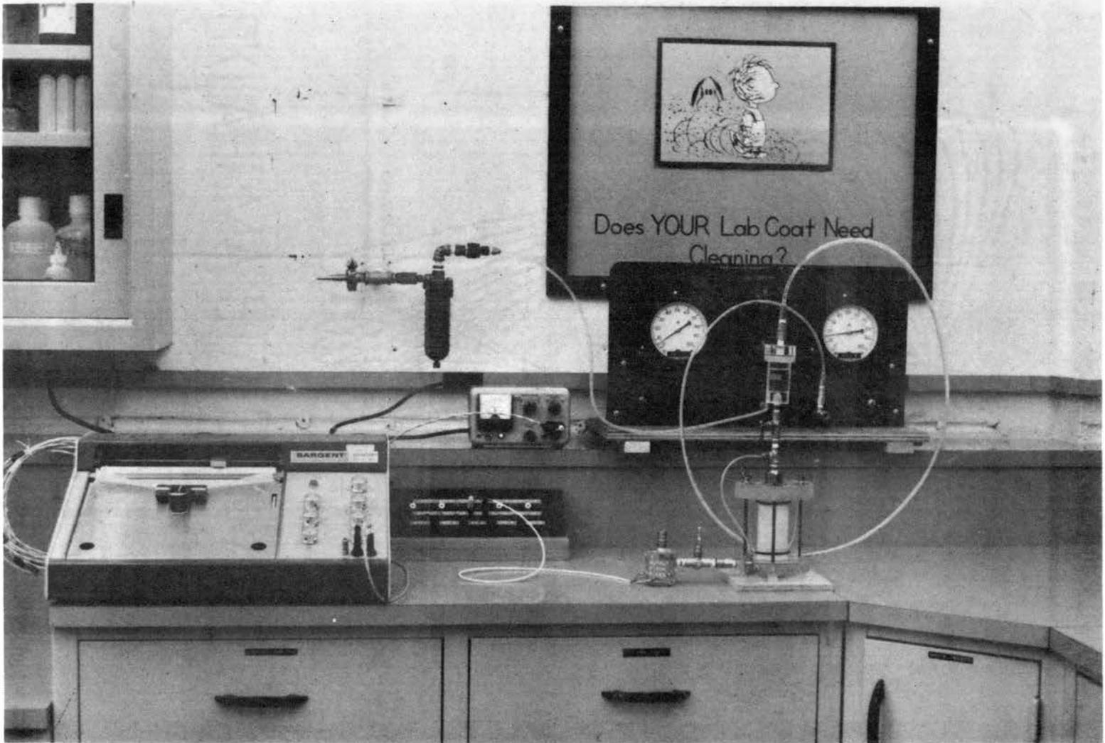
Figure 3.5. Test Assembly for Lateral Swelling Pressure Measurement.
