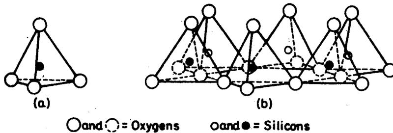
Figure 2.1. Diagrammatic Sketch Showing (a) a Single Silica Tetrahedron and (b) the Sheet Structure of the Silica Tetrahedrons (after Grim, 1968).
