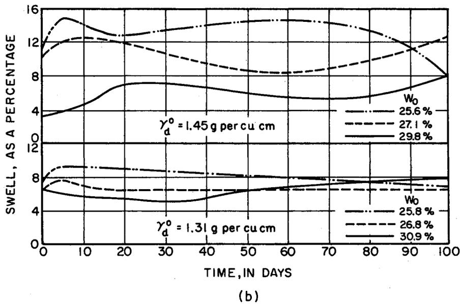
Figure 2.13. Effect of Curing Period on (a) Swelling Pressure and (b) Swell (after Kassif and Baker, 1971).
