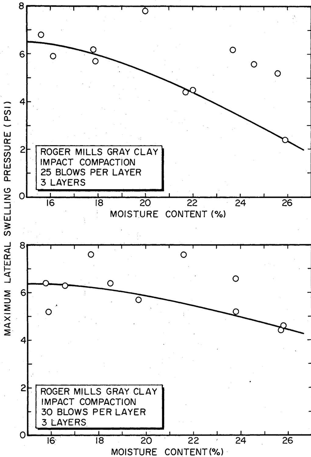
Figure 4.4. Effect of Initial Moisture Content on Lateral Swelling Pressure for RMGC.
