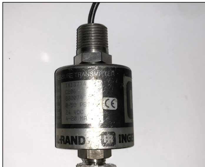
Figure 29 Pump discharge pressure transducer
