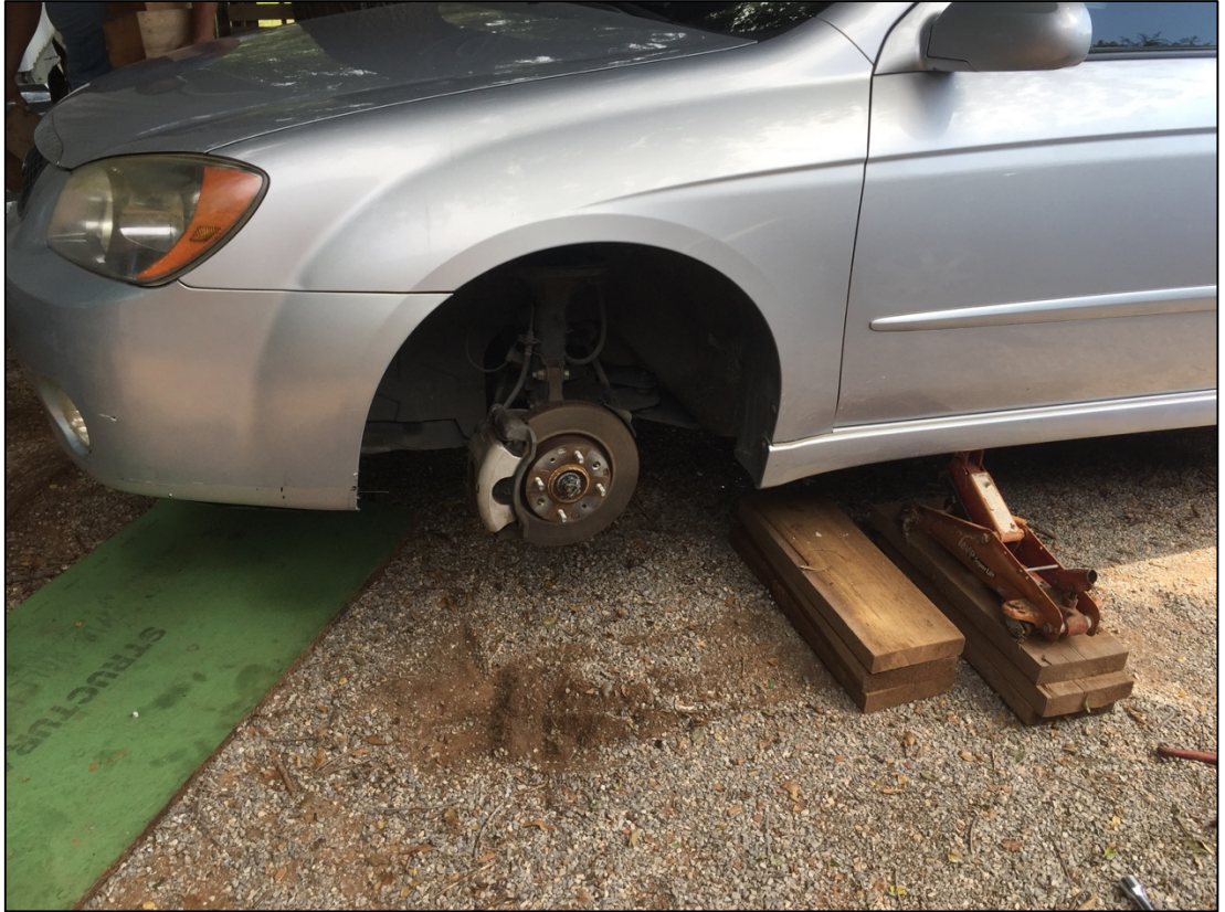
Figure 8. The Broken Jack and Piles of Lumbers Used as Jack-Stands.
