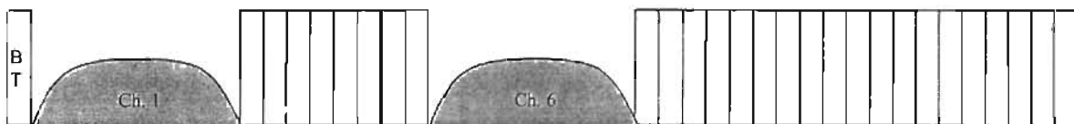
Figure 5.6 Frequency Overlap between IEEE 802.11 Channel 1 and 6 and Bluetooth Spectrum
