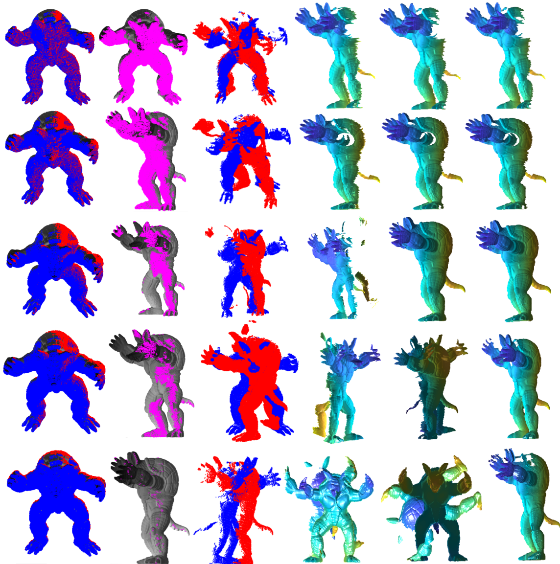
Figure 7.4: Results from Table 1 : Rows ( 30^\circ, 60^\circ, 90^\circ, 120^\circ, 160^\circ ), Columns (Two original range scan data, overlapping area(magenta), initial pose from the depth camera, M-ICC, PA-MMICC, AS-MMICC algorithm results, respectively).
