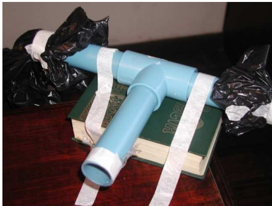
Fig 1. T-maze with choice chambers as dark plastic bags (containing paper towels conditioned by mother) into which the test L. leopardinus neonate falls and cannot reverse its decision.
