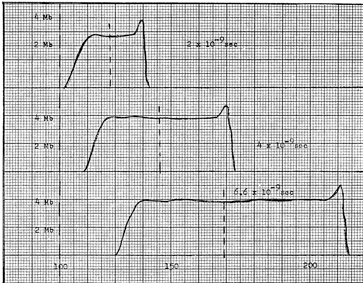
Figure 31. Pressure Profiles Resulting from Impact of Iron Plate of Porosity 1.33 Traveling at 15.2 Km/sec
