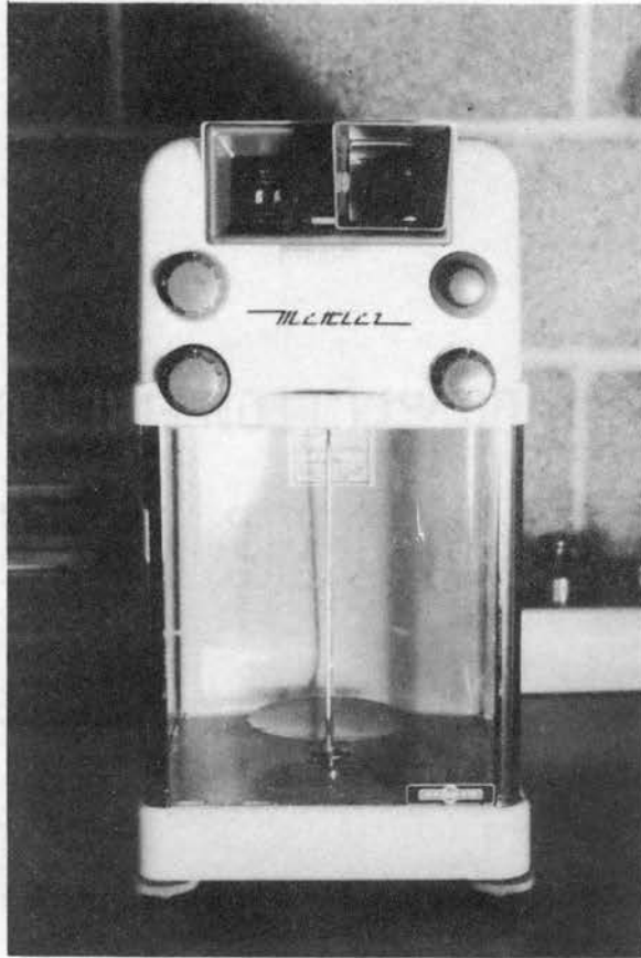
Figure 5. Mettler analytical balance, Type H16, used in weighing pupae.
