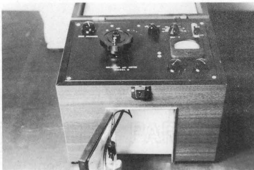
Figure 4. Beckman, Model G, pH meter used in determining hydrogen ion concentration (pH) of diets.
