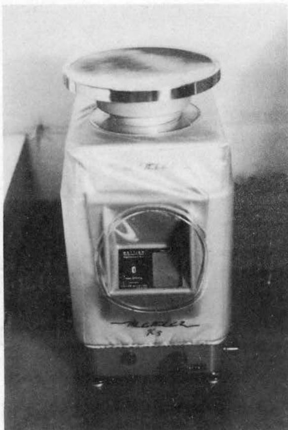
Figure 2. Mettler balance, Type K5, used in weighing dry constituents of diets.
