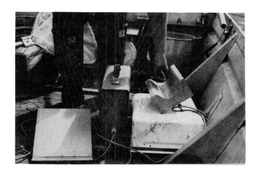
study was U-shaped which permits usage with fish of any size. When the head of a fish containing a magnetized metal tag was moved rapidly past the sensing head at a distance of about 1-10 cm, the audio unit emmitted an audible response.
