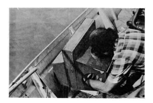
Figure 5. Use of a U-shaped sensing head and connecting detector to determine presence of a magnetic nose tag in fish.
