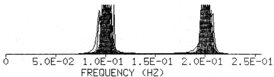
Figure 26. 1-D LP ( L_2 Norm) Spectral Estimate ( N = 8 ; f_1, f_2 = .1, .2 Hz; 30 dB Gaussian noise; 100 Monte Carlo trials)
