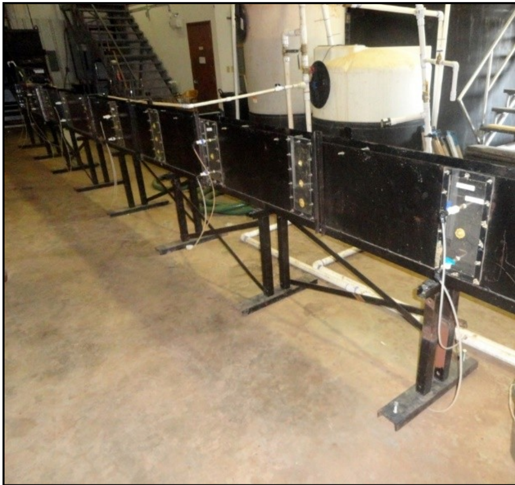
Figure 3.9. Flume apparatus used for determination of flocculation efficiency.
