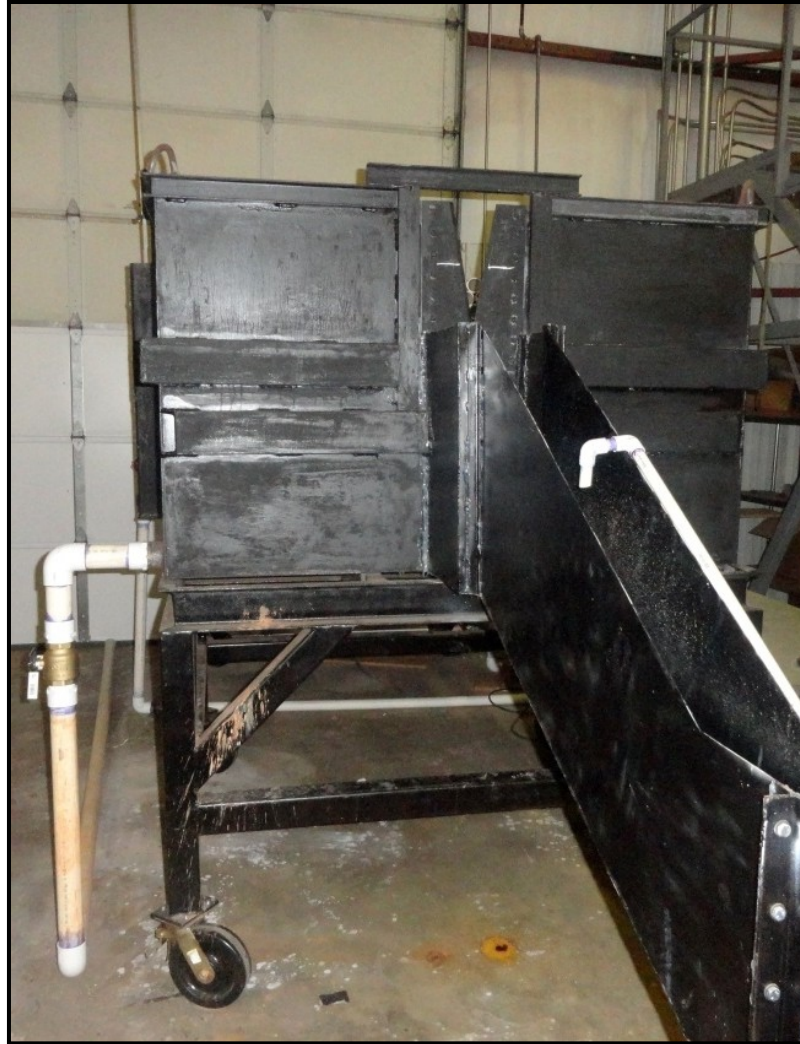
Figure 3.6. Constant head tank as constructed for regulating flow into the flume.
