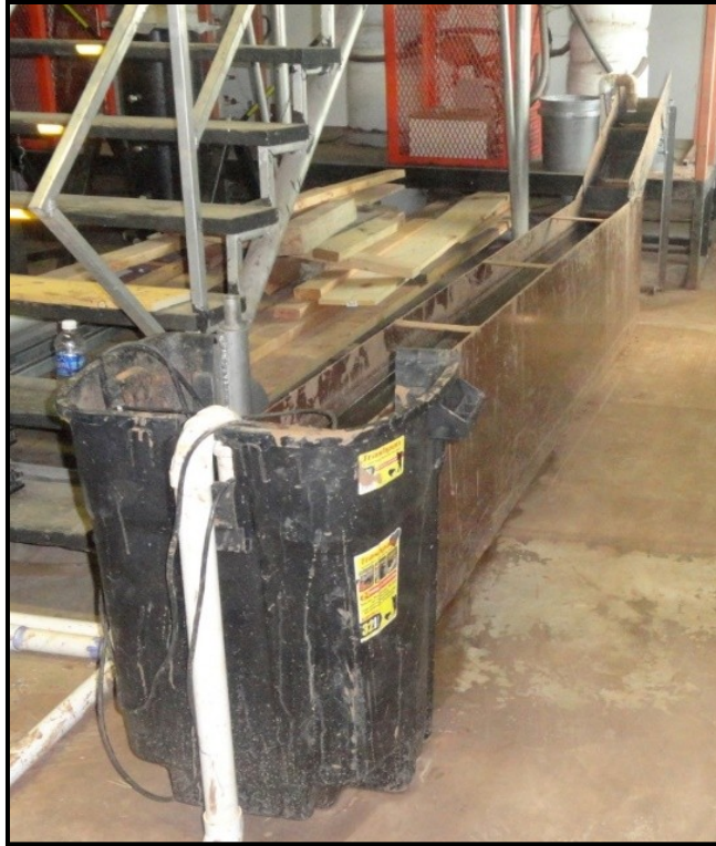
Figure 3.1. Soil separator used to remove sand particles and large aggregates.
