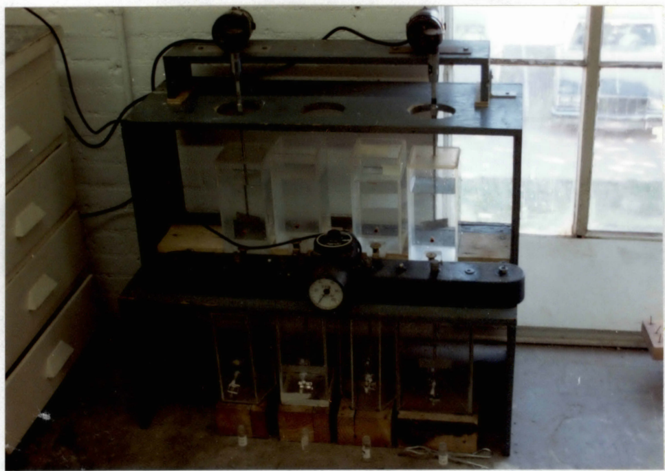
Figure 37. Photograph showing the arrangement of Rapid and Slow Mix Set Ups.
