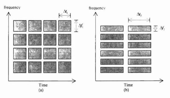
Figure 2-1: Decomposition of signal using STFT (a) long analysis window function, (b) short analysis window function.
