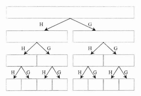
Figure. 2-11: Implementation of discrete wavelet packet decomposition
