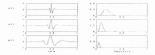
Figure 2-6: Wavelet basis function and corresponding frequency spectrum. The frequency axis is in units of  $\pi \times$  radians.
