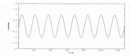
Figure 2-16: A signal localized in frequency domain
