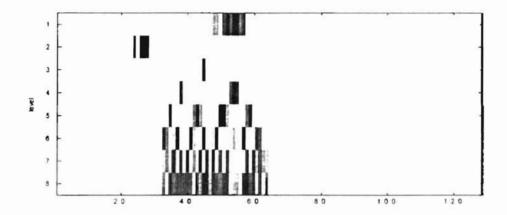
Figure 2-19: The WPD image representation of a time and frequency localized signal
