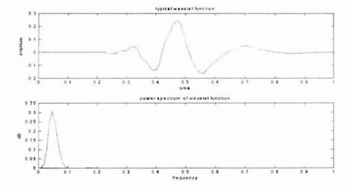
Figure 2-5: A typical wavelet function and its spectra. The frequency axis is in units of  $\pi \times$  radians.
