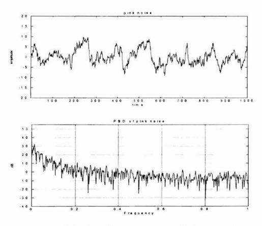
Figure 4-4: Pink noise and its power spectrum. The frequency axis is in units of  $\pi \times$  radians.
