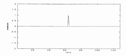
Figure 2-14: A signal localized in time domain
