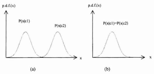
Figure 3-5: Probability density functions of (a) two well separated classes and (b) two completely overlapping classes
