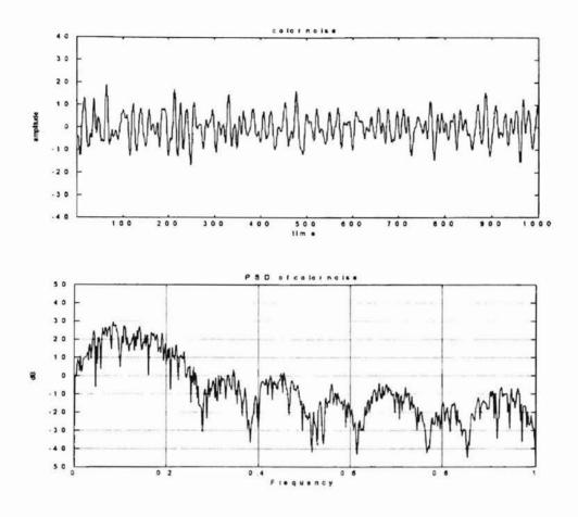
Figure 4-3: Color noise and its power spectrum. The frequency axis is in units of  $\pi \times$  radians.
