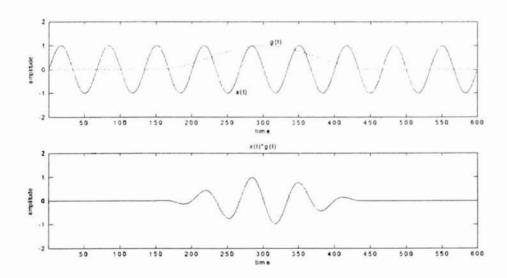
Figure 2-2: Proper analysis window function
