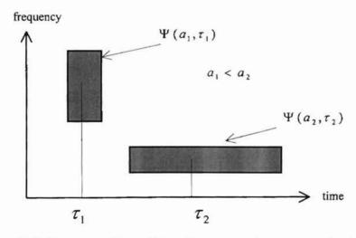
Figure 2-7: Decomposition of signal using continuous wavelet transform
