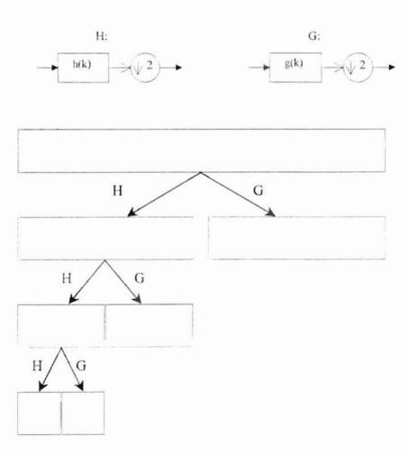
Figure. 2-9: Implementation of fast wavelet transform
