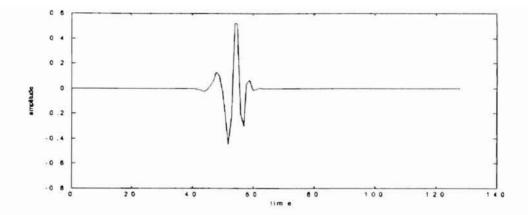
Figure 2-18: A signal localized in both time and frequency domain
