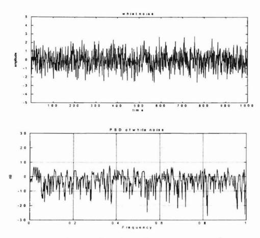
Figure 4-2: White Gaussian noise and its power spectrum. The frequency axis is in units of  $\pi \times$  radians.
