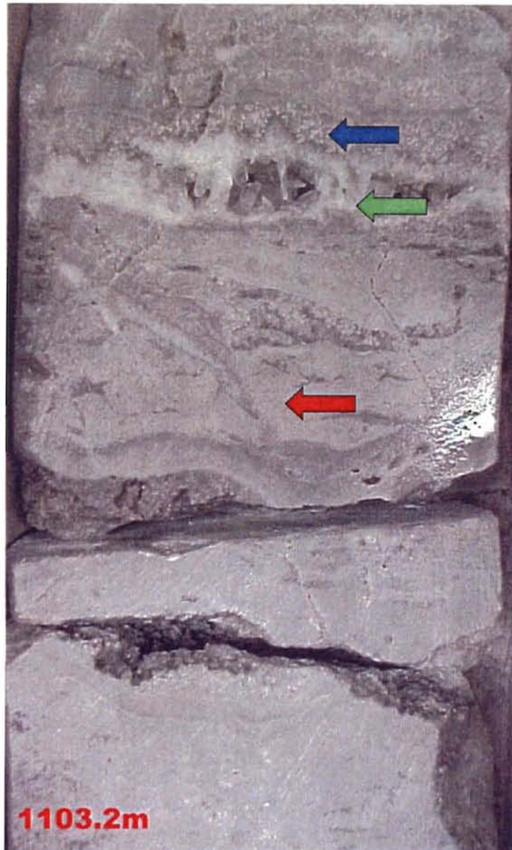
Figure 26. Core photo of the shallow stromatoporoid bank facies with large calcite filled vug (green) within tabular stromatoporoids (red) and renalcis (blue). CZAR b-66-H/94 P 10, depth 1103m.
