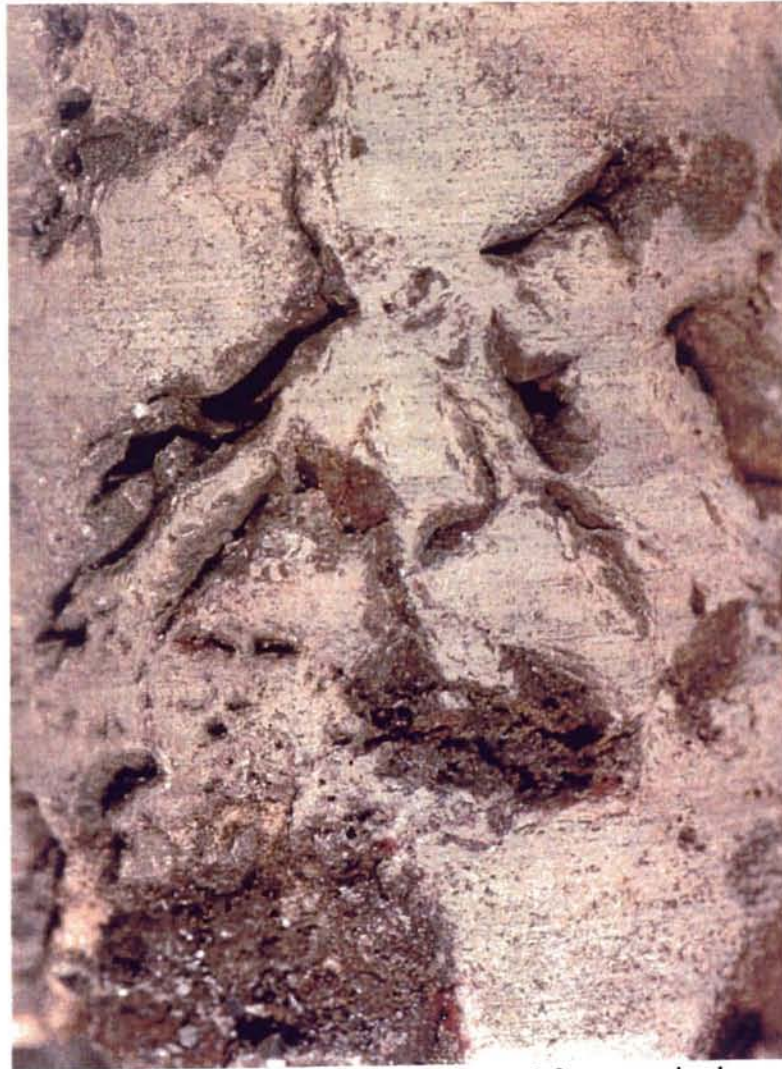
Figure 18. Core photo demonstrating solution enlarged fractures in the c-18-A/94 P 10 at 1134 m.
