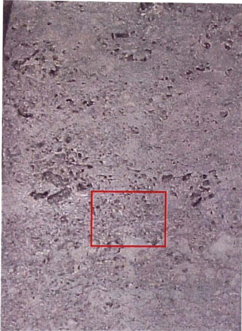
Figure 27. Core photo demonstrating microvugular porosity (red) within the shallow stromatoporoid facies created by the leaching of renalcis . CNRL a-40-A/94P 15, 1131.85 m.
