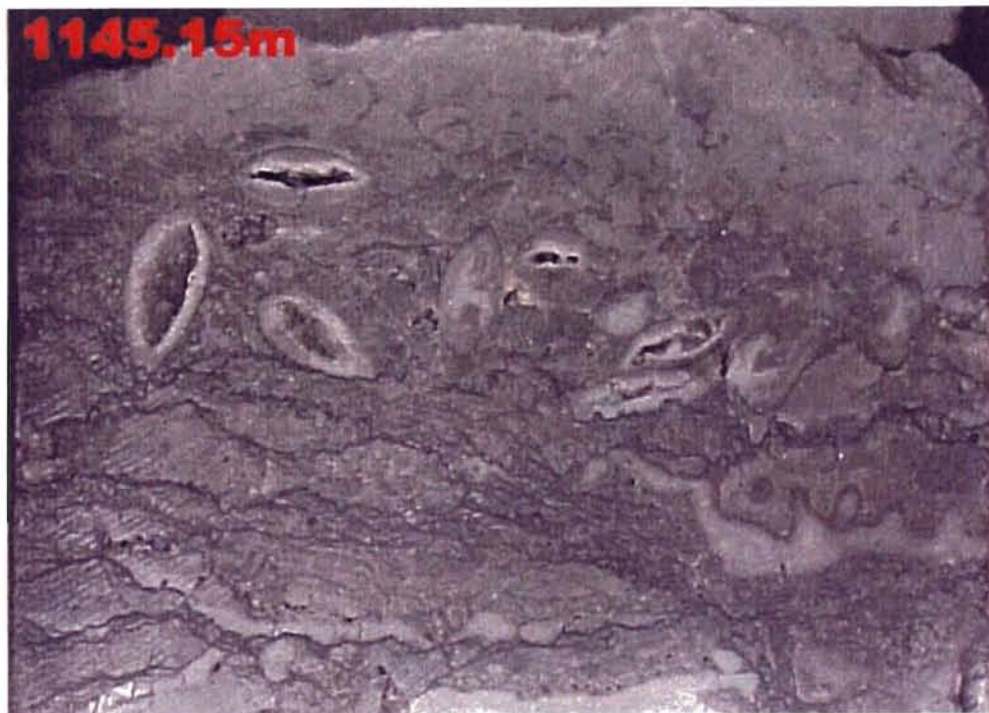
Figure 28. Core photo showing shelter porosity within the marine shelf/amphipora shoal biofacies. Here the shelter is created by large ostracod shells. CZAR d-91-J/94 P 7, 1145.15m.
