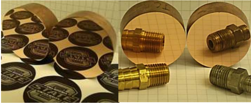
Figure 5.3 Polished blanket copper wafers after 12 min of CMP
