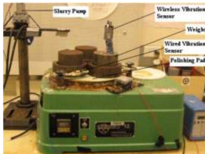
Figure 4.5 Experimental setup using a LapMaster L 12 Bench-top lapping machine.
