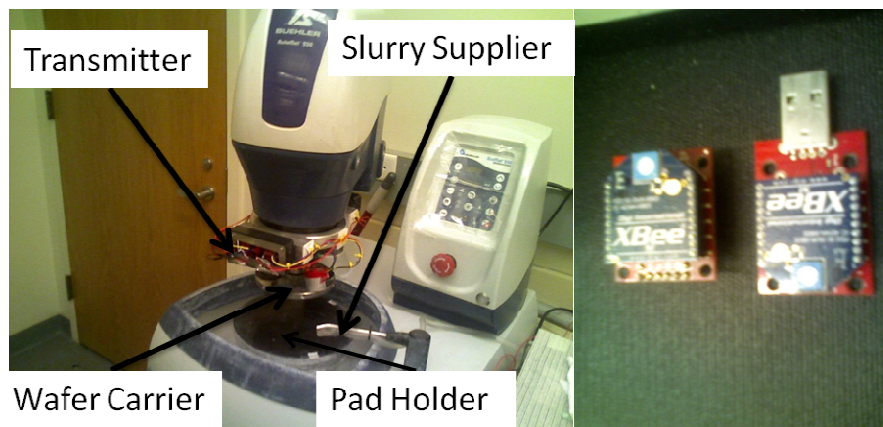
Figure 5.2 Buehler Automet ® 250 experimental CMP polishing setup and wireless Xbee Vibration Sensor
