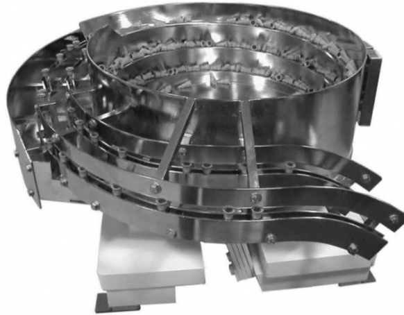
Figure 11. Many industrial part feeders use vibratory or centrifugal force agitation for part positioning and/or orientation. The depicted 21” bowl feeder by Service Engineering, Inc. advances 20 parts per minute to the next processing step. Image by courtesy of Service Engineering, Inc. http://www.serviceengineering.com/
