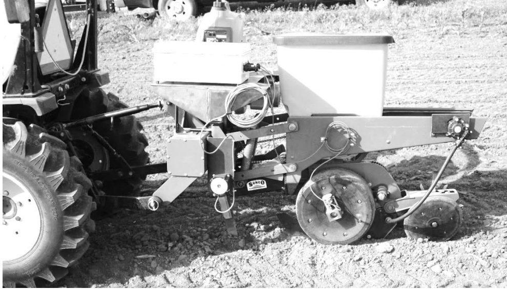
Figure 35. The prototype one-row planter in the field.
