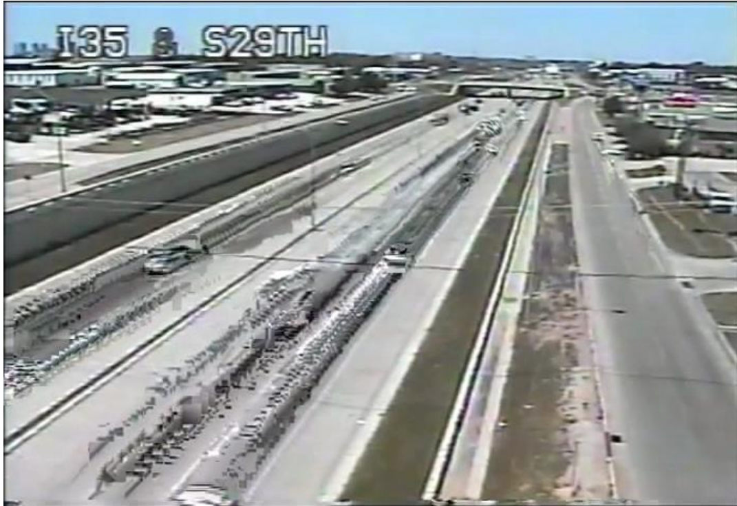
Figure 15. Illustration of pixel errors in actual video from the Oklahoma statewide ITS. The errors are usually rejected to moving object such as vehicles.
