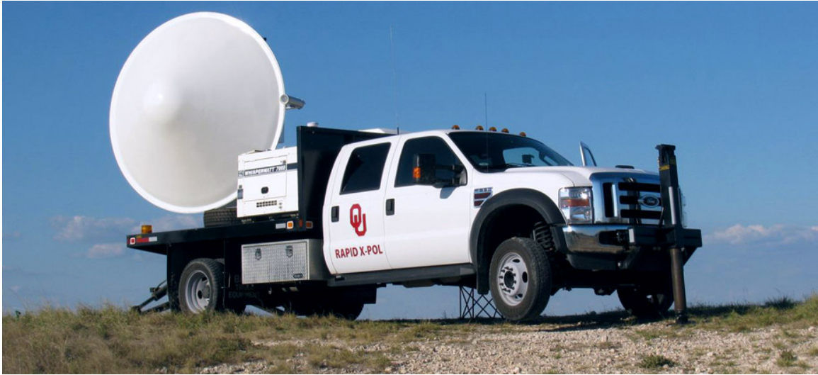
Figure 3.29: RaXPol radar leveled for field experiment. The photo is provided through the courtesy of Dr. Philip Chilson.
