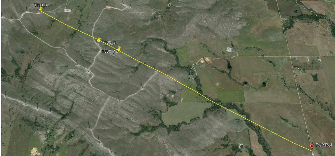
Figure 3.34: RaxPol deployment in the Lawton wind farm. The red pin is RaXPol, and the three yellow ones are wind turbines found along the radar beam. The azimuth steering is 300^\circ from north.
