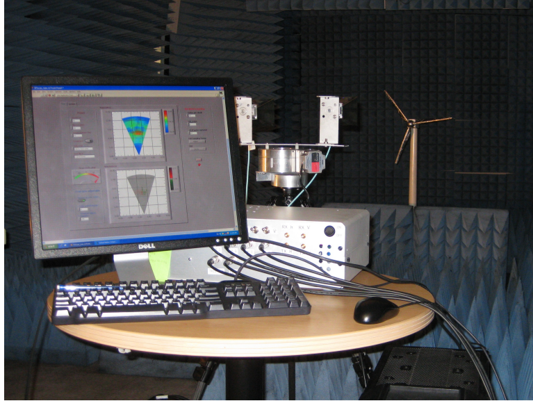
Figure 4.22: Time domain measurement setup. The bottom of the wind turbine model is covered to reduce scattering from the base. The monitor shows the software user interface developed using LabVIEW.
