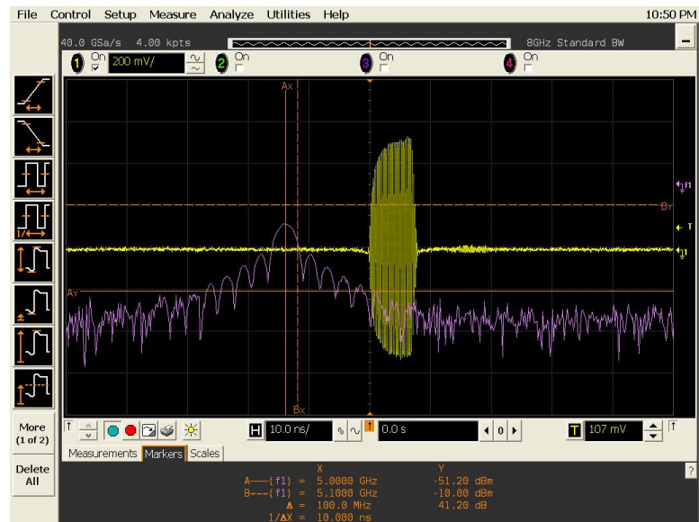
Figure 4.7: Test measurement of the commercial RF switch module. Yellow is output waveform in the time domain and purple is the corresponding Fourier transform. The test was performed at 5 GHz instead of 10.5 GHz as the oscilloscope only supports up to 8 GHz sampling.
