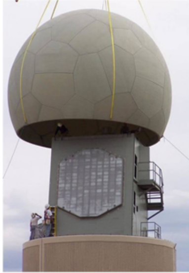
Figure 1.5: The Phase Array Radar in Norman, Oklahoma. The array antenna is from military radar AN/SPY-1A. PAR is the key instrument of the National Severe Storm Laboratory (NSSL) weather radar testbed for developing new algorithms and investigating the feasibility of multi-mission phase array radar. Photo is provided through the courtesy of A. Zahrai.
