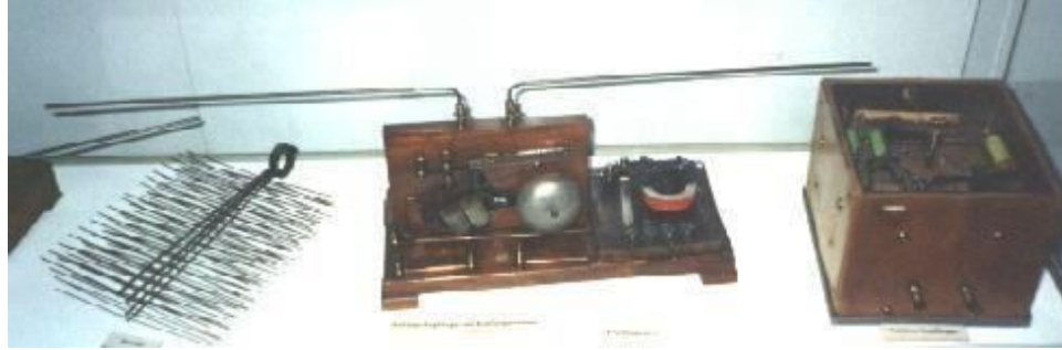
Figure 1.1: Christian Huelsmeyer's invention of "telemobiloscope" displayed at the Deutsches Museum in Munich. The antenna is on the left, the receiver in the middle, and the transmitter is on the right. If a target is detected, the bell keeps ringing until it moves out of the field-of-view. The detecting range is 3000 m. Picture from the "RADAR WORLD" http://www.radarworld.org/huelsmeyer.html .
