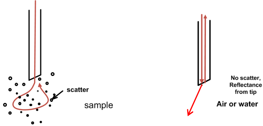
Fig. 3.7 Illustration of reflectance from scattering medium and non scattering medium
