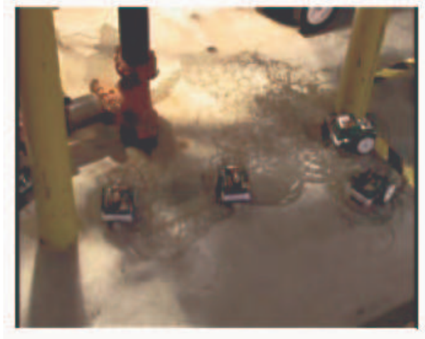
Figure 2.12: Robots deployed in a cluttered DOE facility form a perimeter around a water spill [2].
