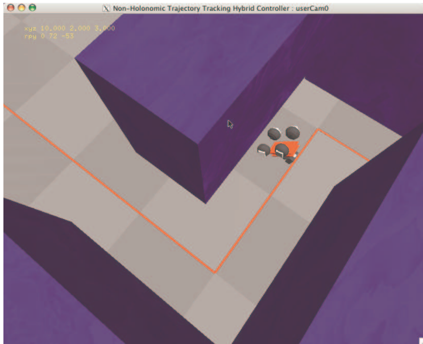
Figure 4.10: Gazebo simulation showing a robot hitting a wall and flipping over.
