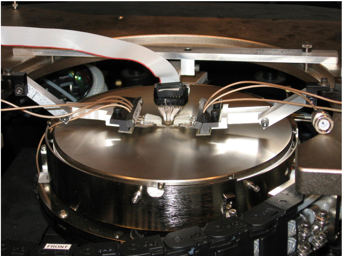
Figure 5.3 Snap of the die on probe station with probes landed
