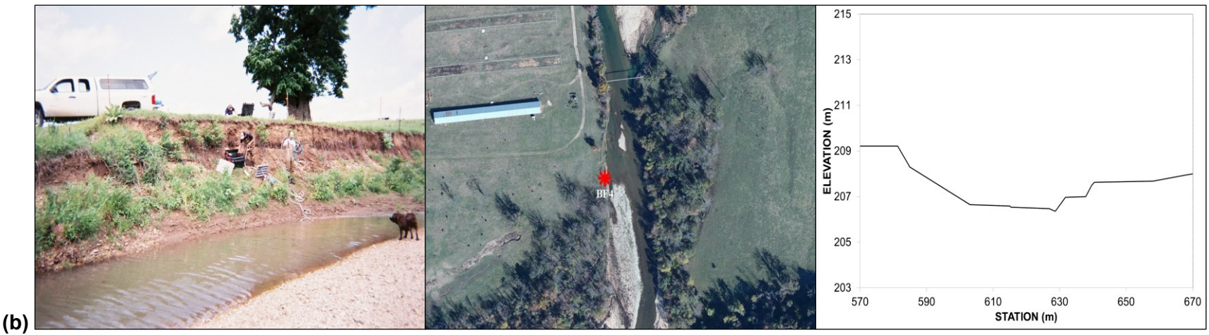
Figure 3-3b. Ground-based photograph, aerial imagery (USDA-FSA, 2010, 1:2000), and initial cross sectional survey at site (a) BF3 and (b) BF4.
