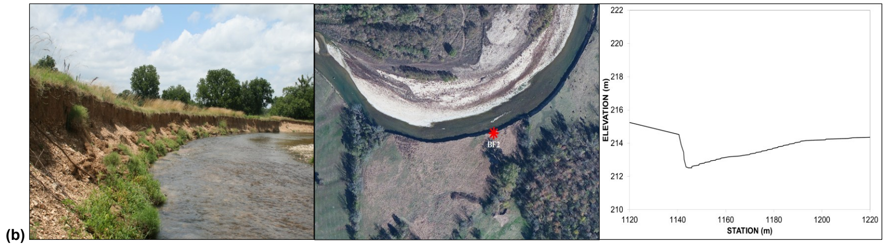
Figure 3-3a. Ground-based photograph, aerial imagery (USDA-FSA, 2010, 1:2000), and initial cross sectional survey at site (a) BF1 and (b) BF2.
