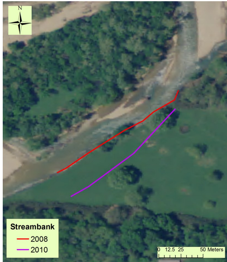
Figure 4-7. Lateral retreat of critical bank near site BF3 on the Barren Fork Creek from 2008 to 2010 displayed on 2008 NAIP imagery (USDA-FSA, 2008).
