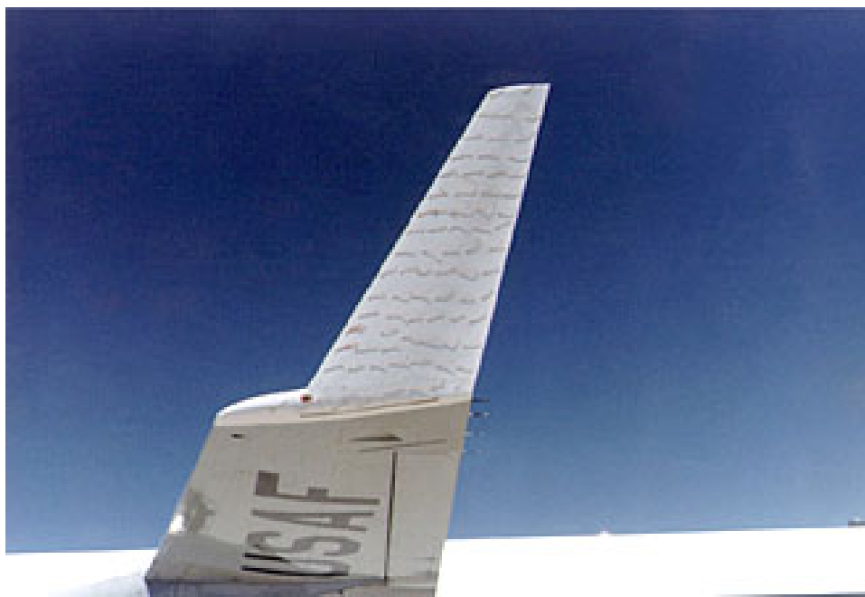
Figure 1.1: In 1979, NASA attached a winglet to a KC135 to evaluate its performance as part of their early winglet research efforts. [21]
