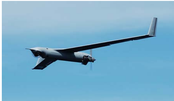
Figure 1.9: The ScanEagle UAV developed by Insitu has a wingspan of 10.2 feet. It is launched using a catapult system, so it doesn't need a runway.[13]
