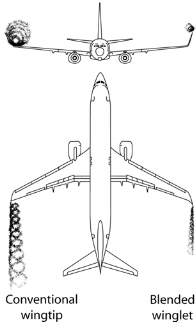
Figure 1.6: Winglets help improve the aerodynamic efficiency by reducing the size of the wing tip vortex.[30]
