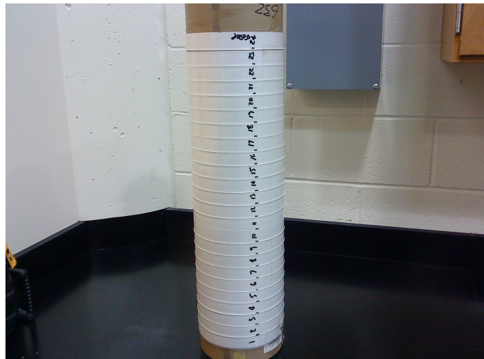
Figure 8.50 Sliced Specimen for Length Measurement
