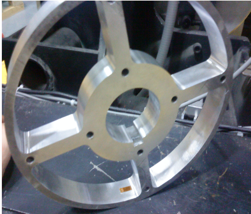
Figure 8.1 7075 Aluminum Segment with Strain Gage Attached
