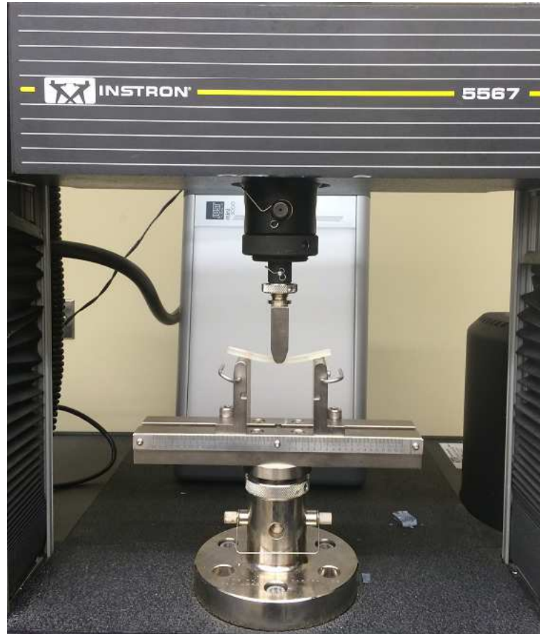
Figure 2.6. Three point bend test of epoxy nanocomposite at span length of 65mm.
