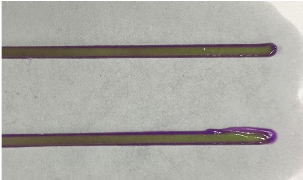
Figure 68: Closeup Image of 150 mm/s and 5 psi Print Condition
