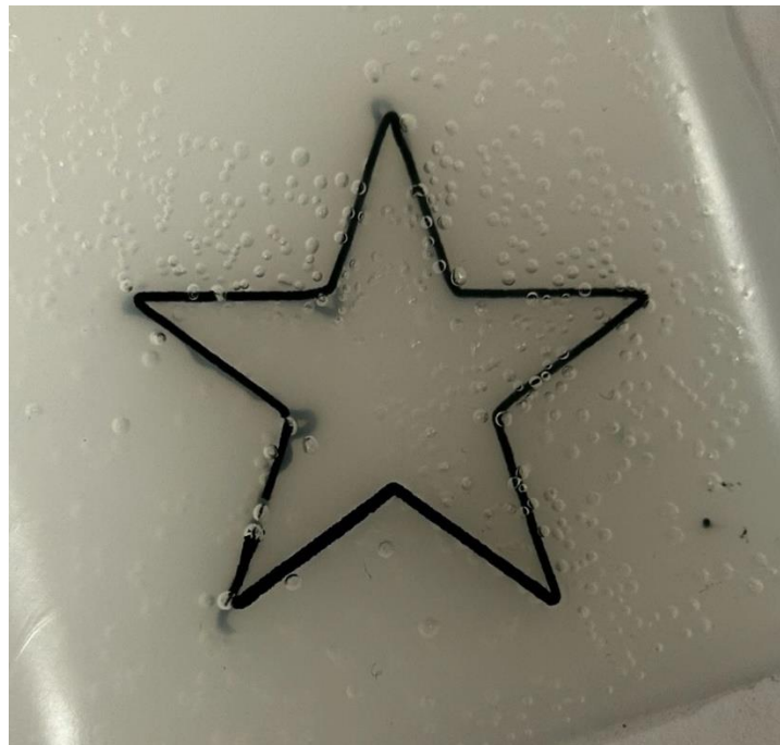
Figure 8: Star Print Attempt with Correct Pressure
