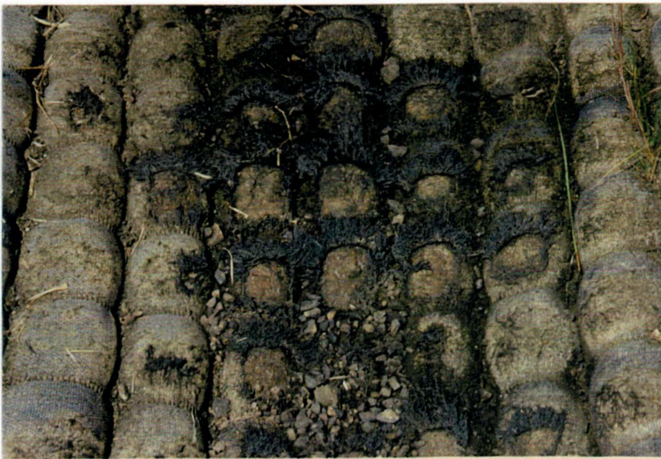
Illustration 8 Showing wear (Polypropylene type)
