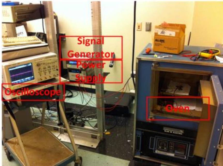
Figure 4.11 Experimental setup for saline test of BP amplifier
