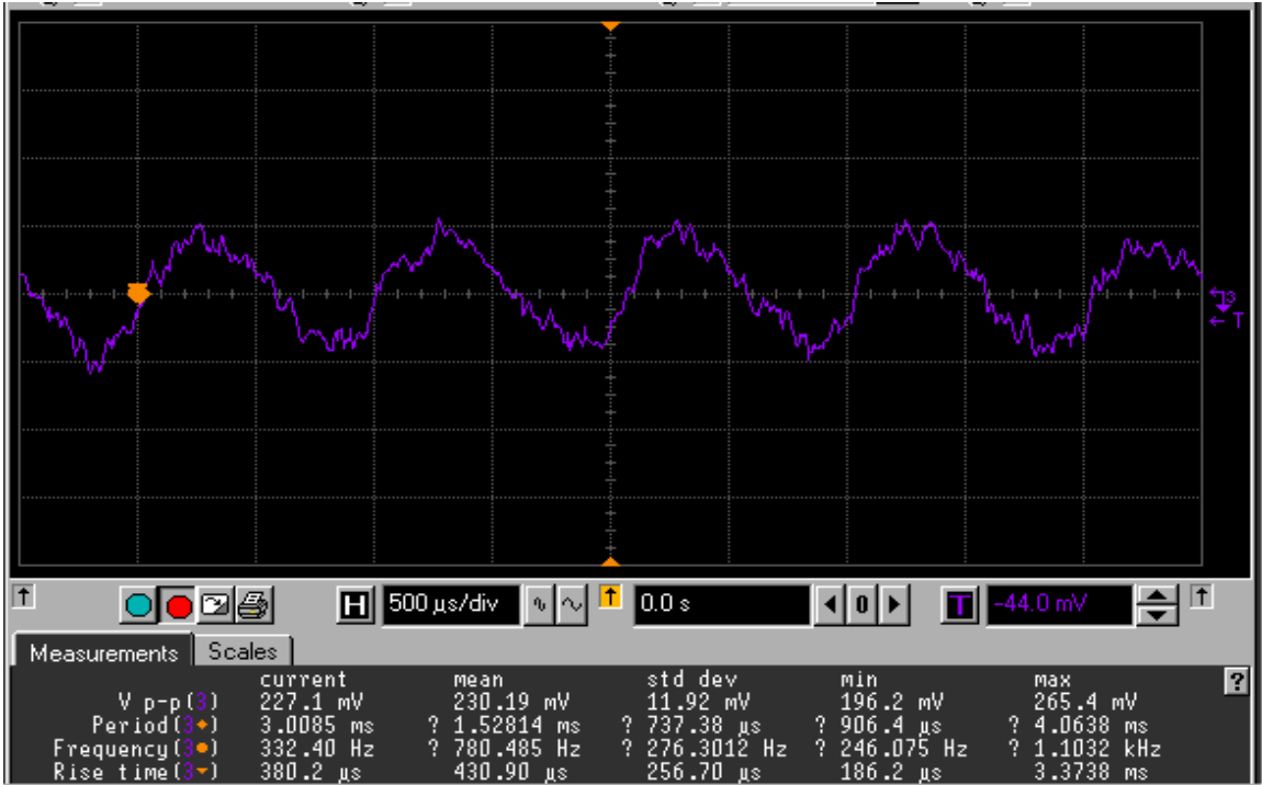
Figure 4.13 Output sinusoid signal when sensed input equals 240uV@1kHz in saline solution
